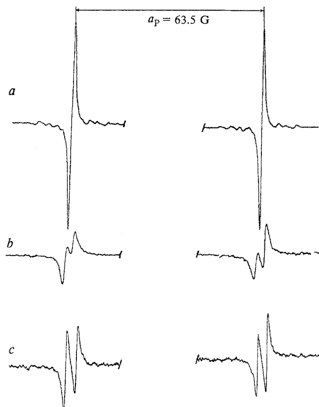
Fig. 2. ESR spectrum of the radical \cdot\text{C}_{60}\text{-P(O)(OPri)}_2 at 300 K (a), 233 K (b), and 200 K (c).
